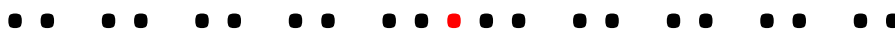
Fig. 6 Images the pattern caused by monochrome light through a slide with multiple slits
